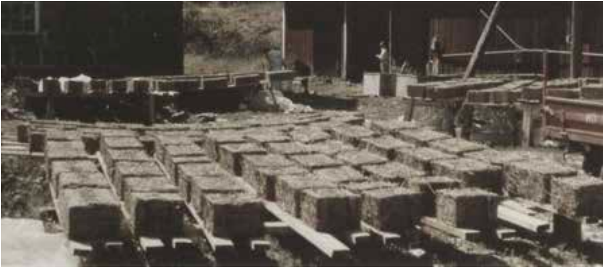
Figure 7: Earth Blocks Drying In The Sun.
