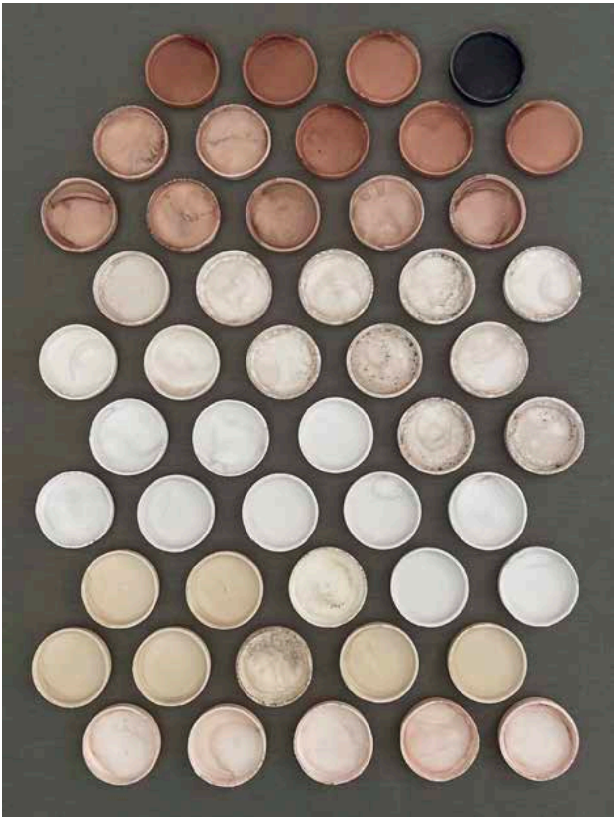
Soil colour samples made from clay. Colours are based upon the averages of all rammed earth destinations visited.
